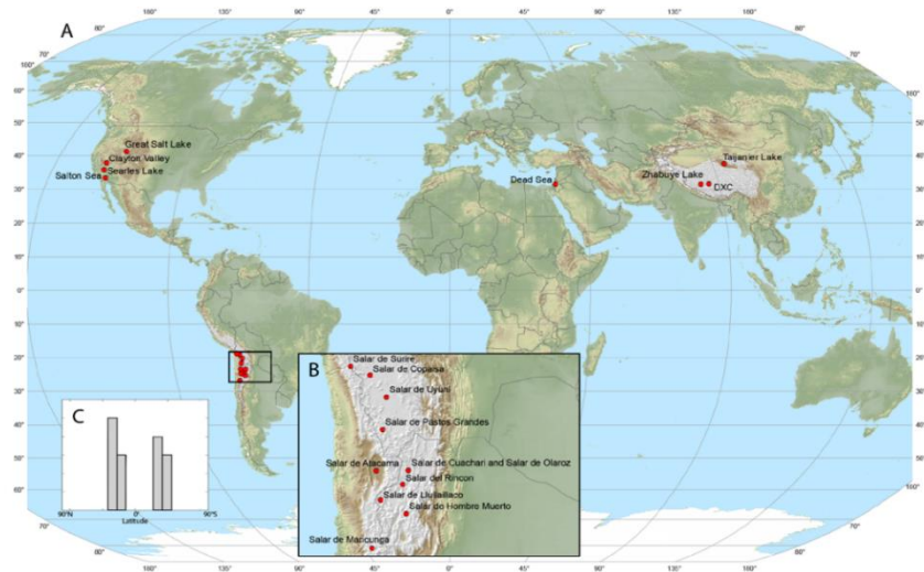
Figure 2. (A) World map of lithium brine deposits (red dots). (B) Detail in South America. (C) Histogram showing the bimodal latitudinal distribution of Li brine deposits in northern and southern arid belts.
